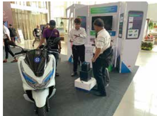
Honda PCX Electric - Swappable battery electric motorcycle
